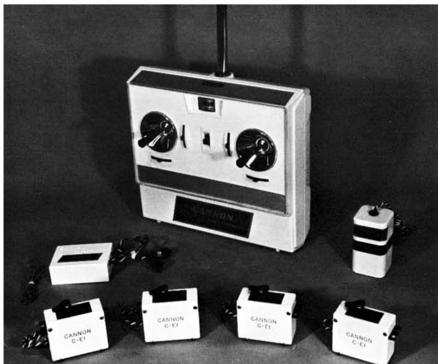
The Cannon Model SP550 Executive IV, a four servo Digital Proportional system to bend your mind. Offered in Mode I or Mode II. Transmitter in background, receiver and battery pack standing. Four servos in the foreground. A rotary type output arm. In 27 mc frequencies.
